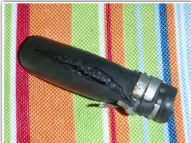
This is what caused the problem - a ruptured coolant by-pass hose located at the back of the engine, up against the firewall.
