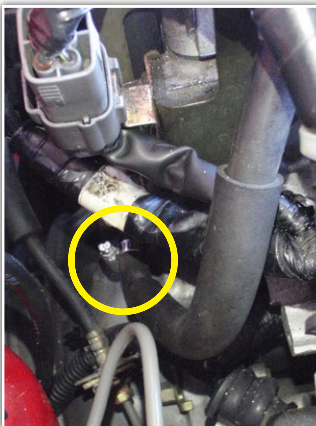
Back of the engine - the rupture happened close to where the bottom clamp is now fitted in this picture. Removing the original spring clip and hose was a nightmare.
