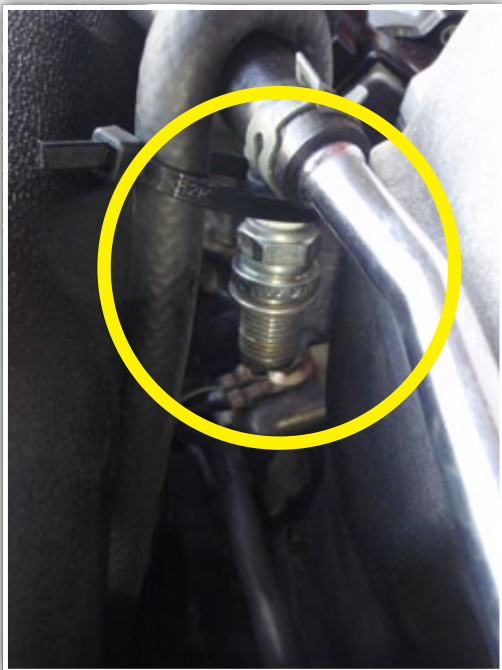
The other bung was an old spark plug, complete with cable tie to hold the hose out of the way. It's agricultural but it worked!
