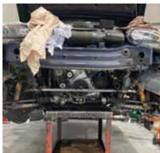
Engine and subframe being fitted to car
